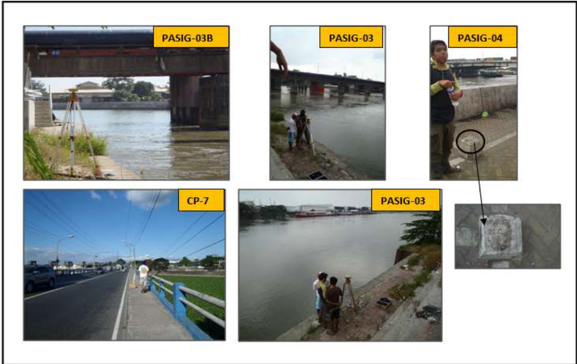
Figure 13. Pictures showing the conduct of GPS observation in some of the control points in Pasig River.
