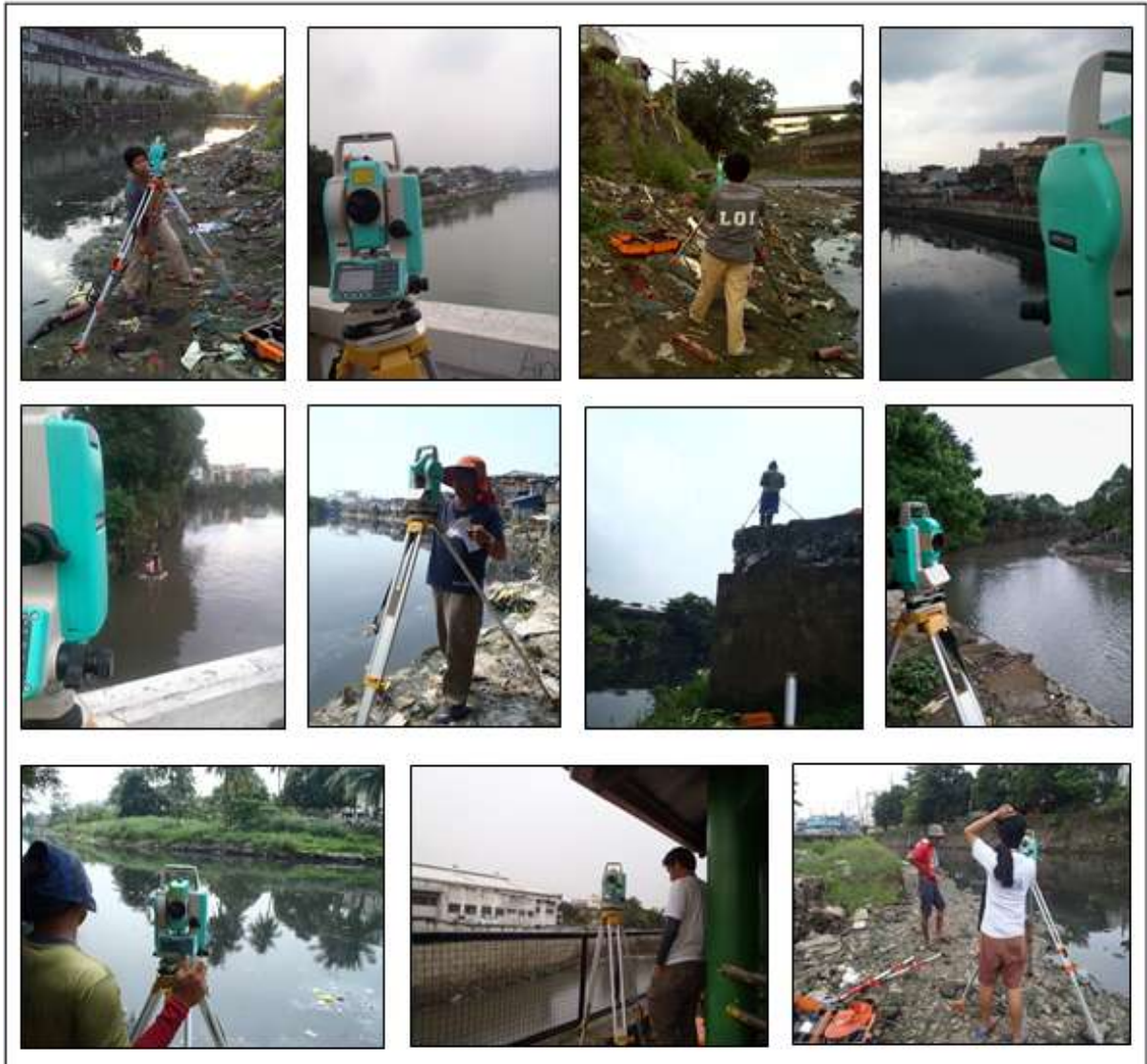
Figure 48. Pictures showing the conduct of profile and cross-section surveys in San Juan River.
