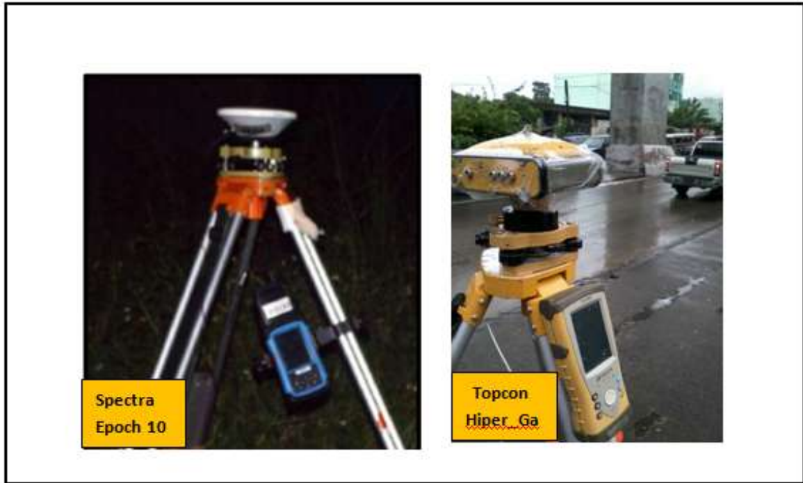
Figure 11. Survey-grade GPS receivers used in getting the horizontal coordinates of the control points.
