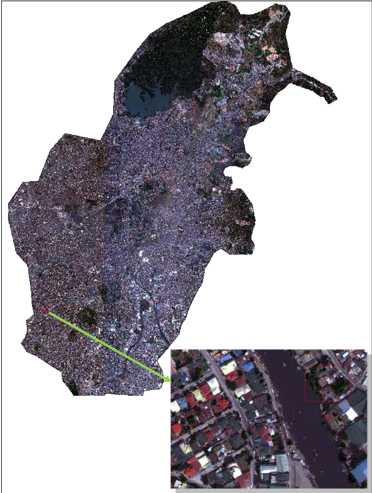
Figure 74. The high resolution WV2 satellite image displayed in true color (RGB = Band 5, Band 3, Band 2). Inset: a close-up view in a portion of the image.
