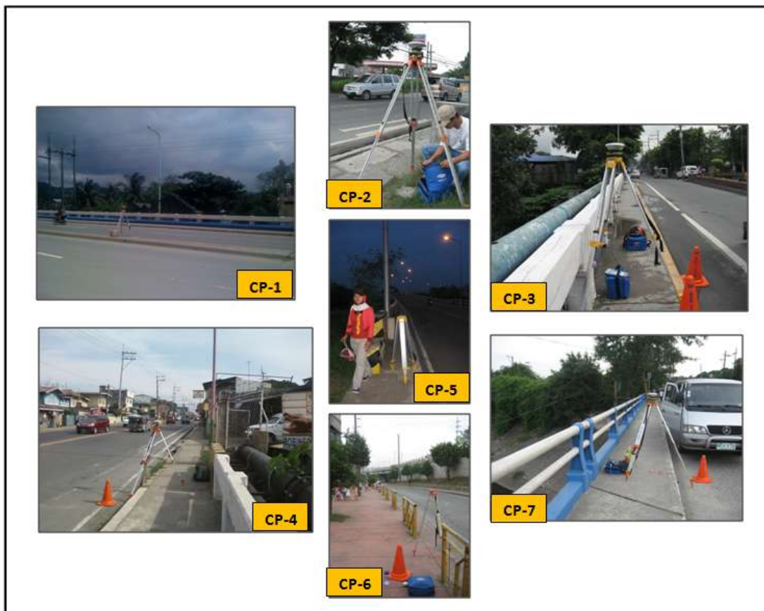
Figure 12. Pictures showing the conduct of GPS observation in some of the control points in Marikina River.
