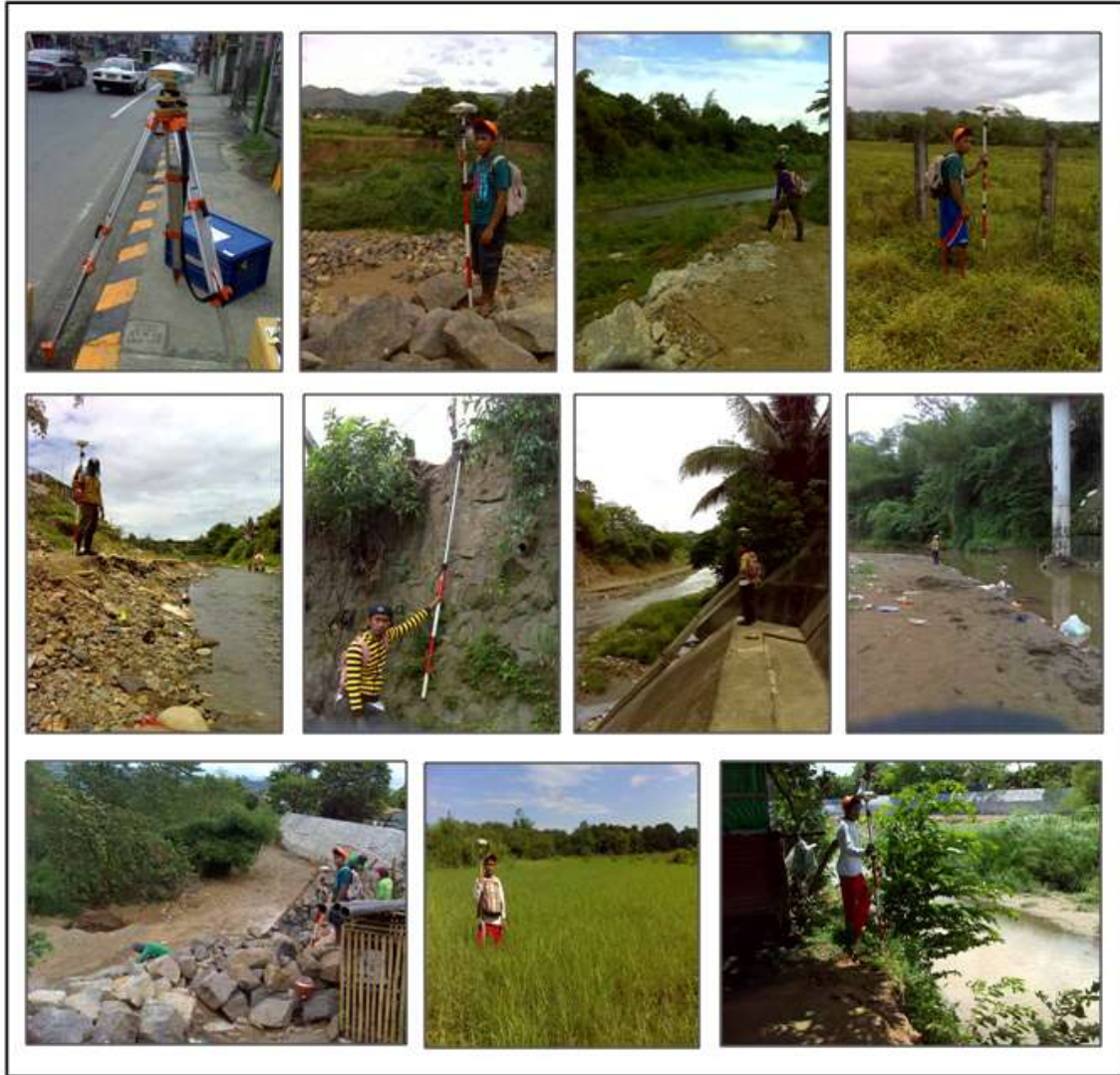
Figure 47. Pictures showing the conduct of profile and cross-section surveys in Nangka River which is a tributary of Marikina River.
