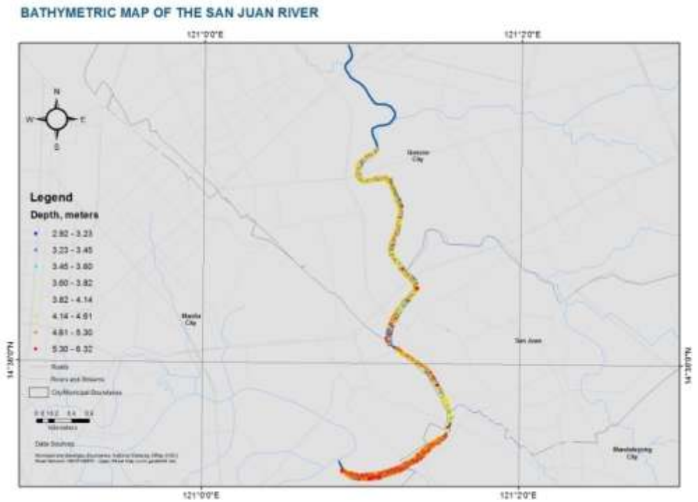
Figure 41. Map showing the bathymetric data points collected using MBES in San Juan River.
