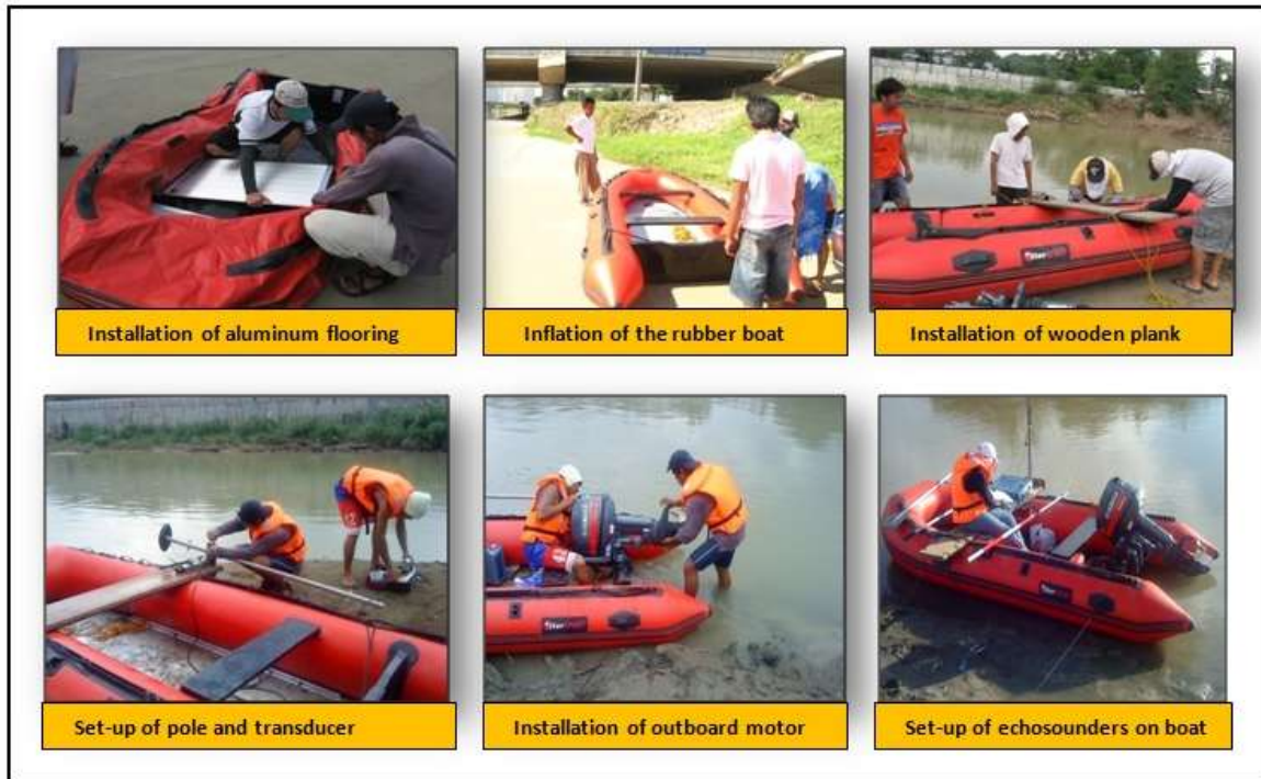
Figure 28. Set-up of rubber boat and echosounders.
