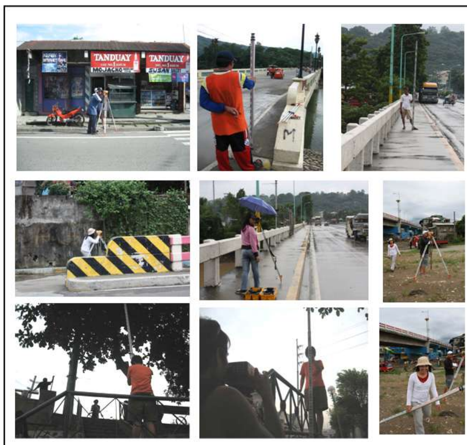
Figure 16. Pictures showing the conduct of 3 rd order leveling surveys in some of the control points in Marikina River.
