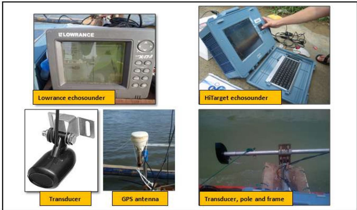
Figure 26. Single-beam echosounders used in the bathymetric surveys of the Marikina and Pasig Rivers.
