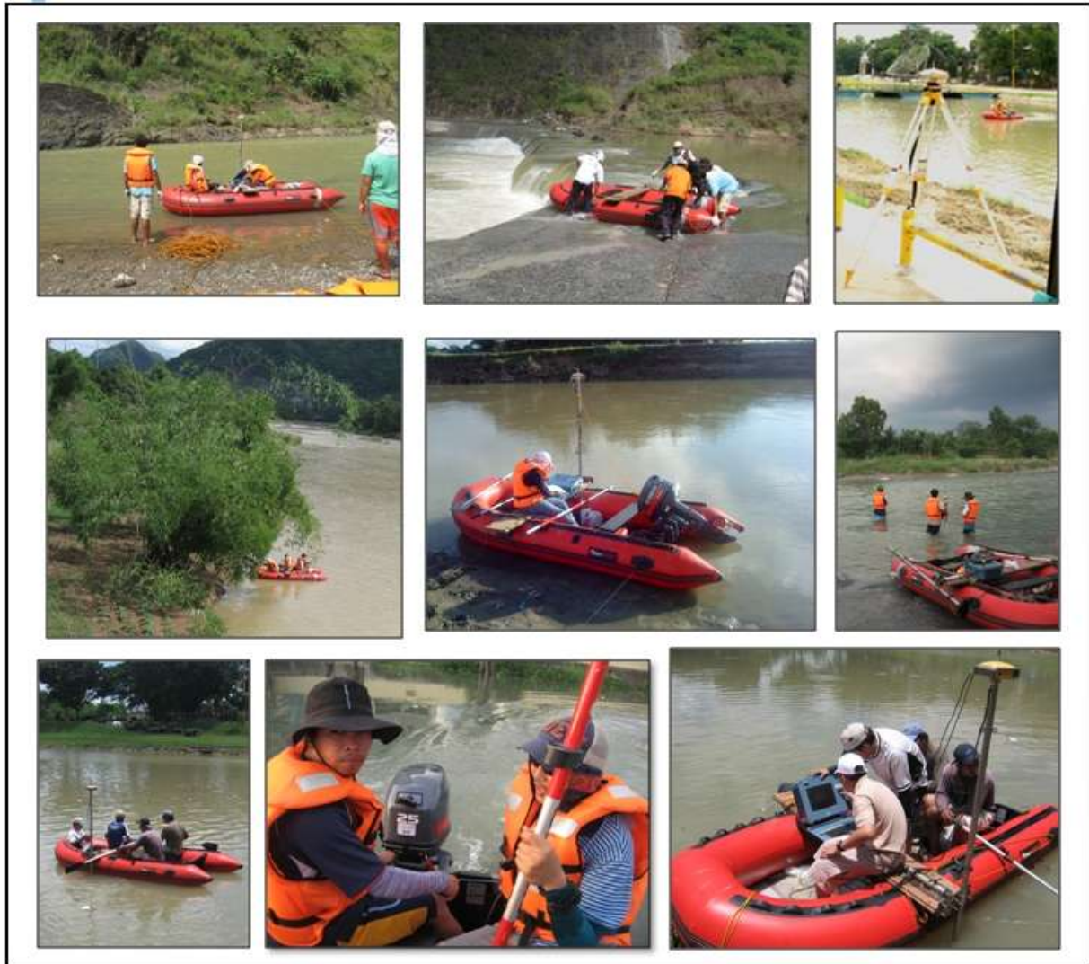
Figure 30. Bathymetric surveys in the Marikina River.
