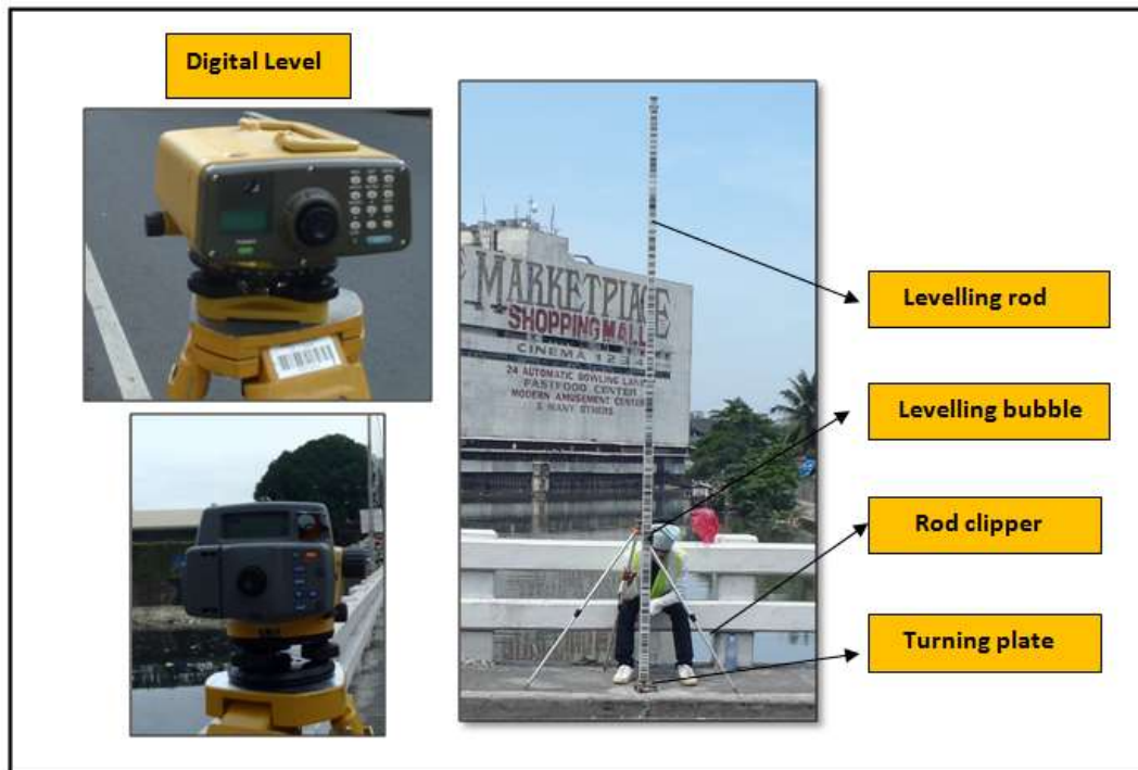
Figure 15. Set-up of equipments for a 3 rd order leveling survey to obtain the MSL elevations of the control points.
