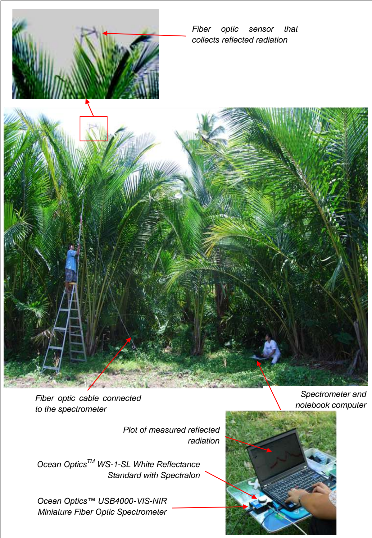
Figure 11. The set-up of the in-situ spectral reflectance measurement conducted in tandem with Sago Project II.2. The set-up is in a stand of Sago palm in rosette stage.
