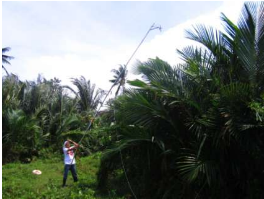
Figure 12. To measure the reflected radiation on top of the Sago palm, the fiber optic sensor is attached to a very long pole.
