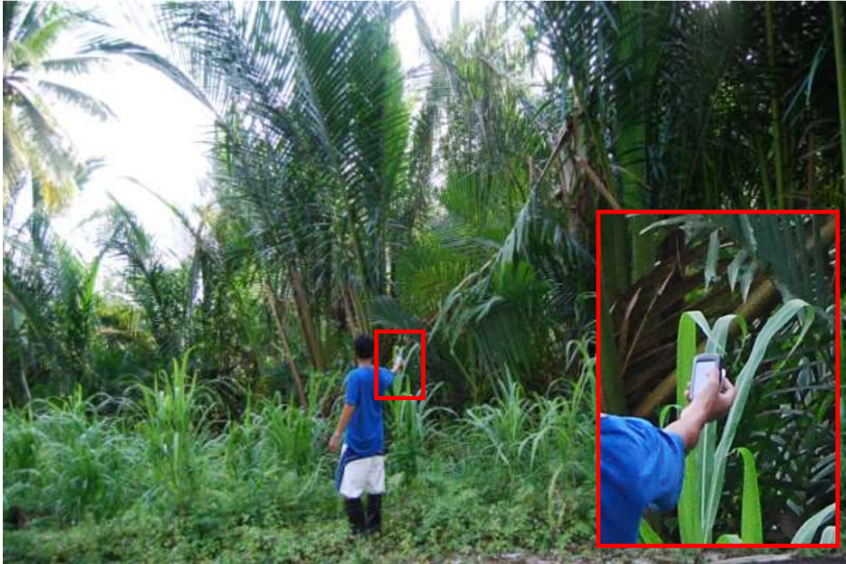
Figure 74. Using the Garmin Oregon 550 GPS to get the perimeter of a Sago palm stand.
